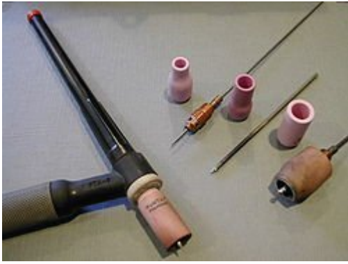
GTAW torch with various electrodes, cups, collets and gas diffusers
